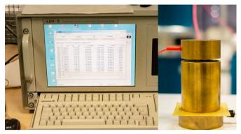
Global method for partial discharge measuring according to IEC 60270
