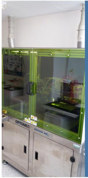
Non-contact deposition of a wide range of organic and inorganic materials, nanocarbon structures and bioactive substances.
